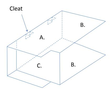
STEP 4 Attach toe kick panel to both side panels using 2 metal cleats and (8)  $\frac{1}{2}$ " flat head screws.
